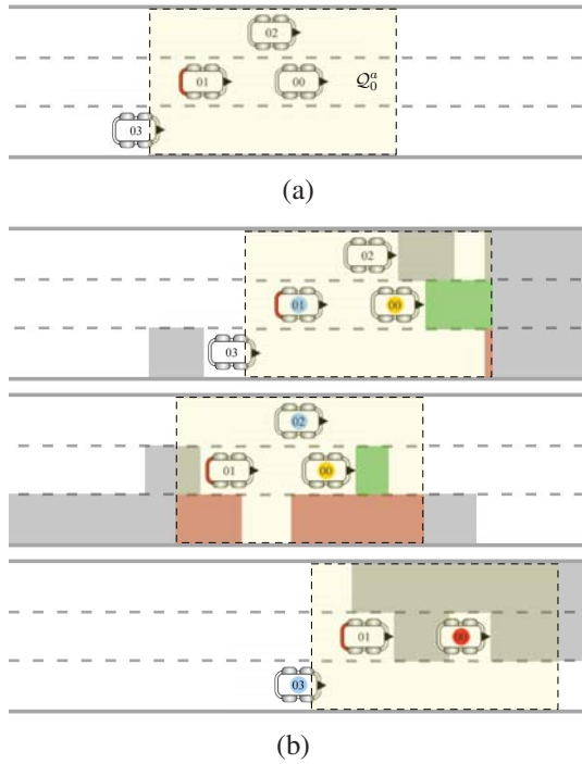
Figure 10. Misbehavior of car 00, running a FAST maneuver along the second lane, while its next right lane is free, has to be detected (a). Local maps of occupancy, M_{00,01} , M_{00,02} , and M_{00,03} , that local monitors on the cars 01, 02, and 03 has reconstructed (b). The yellowish area dashed box outlines the target agent neighborhood; a blue circle specifies the current monitor; red (green) areas are non-visible regions, where the presence (absence) of a car is required. A colored circle around the target robot (green, yellow, or red) specifies its estimated cooperativeness (cooperative, uncertain, or uncooperative, respectively).
