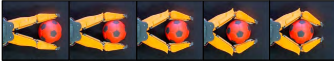
Fig. 5. Pull-in grasping strategy : Depicted is a sequence of intermediate grasp states where the gripper’s belts are used to pull the object towards the palm which results in a transition from a fingertip to an enveloping grasp.
