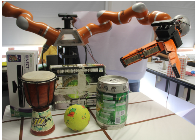
Fig. 1. Platform and test objects : The platform utilized in the test runs in Section IV comprises the Velvet Fingers gripper with three actuated DoF (one for open/close movement and one per finger for conveyor belt actuation) and a seven-DoF KUKA lightweight arm. Perception is done with an ASUS Xtion structured light camera mounted on the gripper. Also shown are the five test objects used in the experiments - two different boxes, a beer barrel, a ball and a drum.
