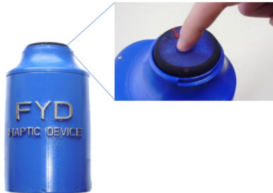
Figure 2.17: The last version of FYD (dimensions: 110 x 90 x 222 mm) and a subject's fingertip interacting with the display.
