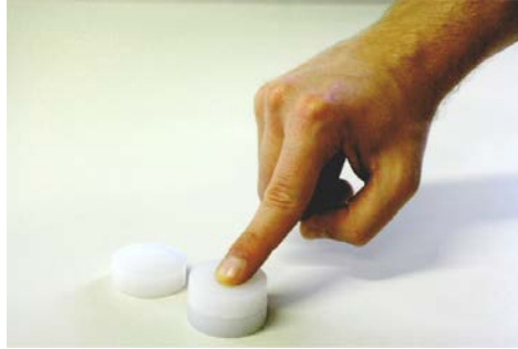
Figure 5.7: A subject's hand palpating one of the silicone specimens used in the tests.
