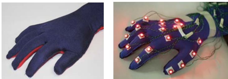
Figure 4.2: The sensing glove by University of Pisa (on the left) and sensing glove with added markers (on the right).
