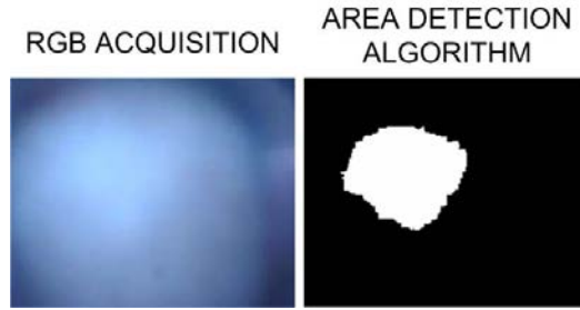
Figure 2.10: The results of the contact area detection algorithm: the RGB acquisition (on the left side) and the result of the final binarization (on the right side).
