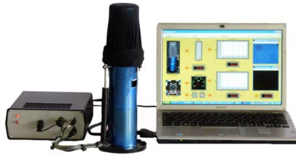
Figure 2.5: The FYD system: starting from the left side, it is possible to see the electronic box, which contains the motor driver and the DAQ card, the FYD prototype and a computer to control the system.
