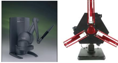
Figure 1.1: Phantom Desktop Device by Sensable (on the left) and Delta Haptic Device by Force Dimension (on the right).
