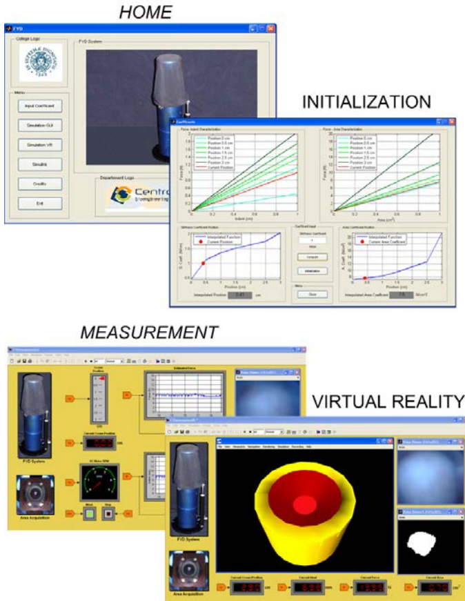
Figure 2.12: GUI: HOME and INITIALIZATION windows for the initialization of the prototype; MEASUREMENT and VIRTUAL REALITY windows to display the values of force, area and indentation.
