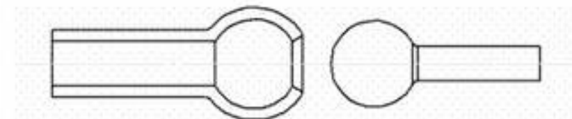
Figure 3: A ball and socket joint is a kind of annular snap fit.
