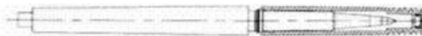
Figure 1: A pen sometimes utilizes an annular snap fit to retain the cap.
