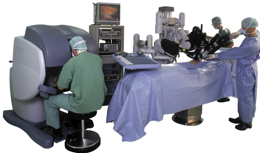
Fig. 1. The da Vinci surgical system. The surgeon operates while seated at the master console. Tools are controlled by translating the surgeon's hand, wrist and finger. Reproduced with permission © 2010 Intuitive Surgical Inc.
